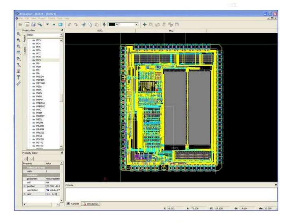
Full-functional layout editor. Set of valid layers defined by technology file and colors defined by packets in DRF file. Each layer has properties like name, number, coordinates.
