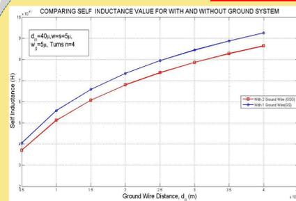
Fig. 3. Comparison Plot of Inductance value for a signal wire with one (GS) and two ground (GSG) system
