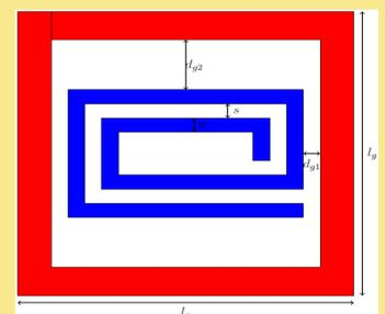
Fig. 7: Rectangular spiral within reference square guard ring area
