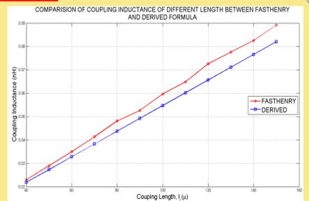
Fig. 4. Coupling Inductance plot for different length of segments of GSG structure
