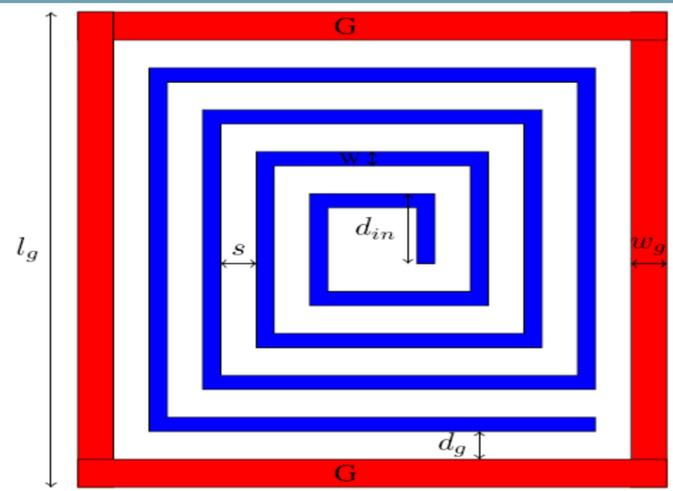
Fig. 1. Basic structure of square spiral inductor with grounded guard-ring for reference
