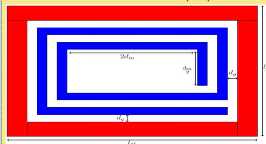
Fig. 6: Rectangular spiral within rectangular guard ring having same area of reference square spiral
