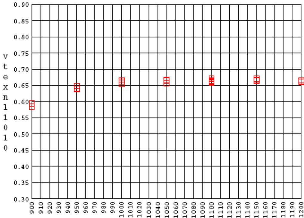
*Dependence of threshold voltage  $V_t$  of 10/10 LVNFET (low-voltage) as a function of field-implant resist thickness ( $P 2.0 \times 10^{13} \text{ cm}^{-2}$  @ 430keV). For resist thickness bellow 1000nm phosphorous implantation penetrates through the resist and oxide underneath, thereby lowering  $V_t$ .*
