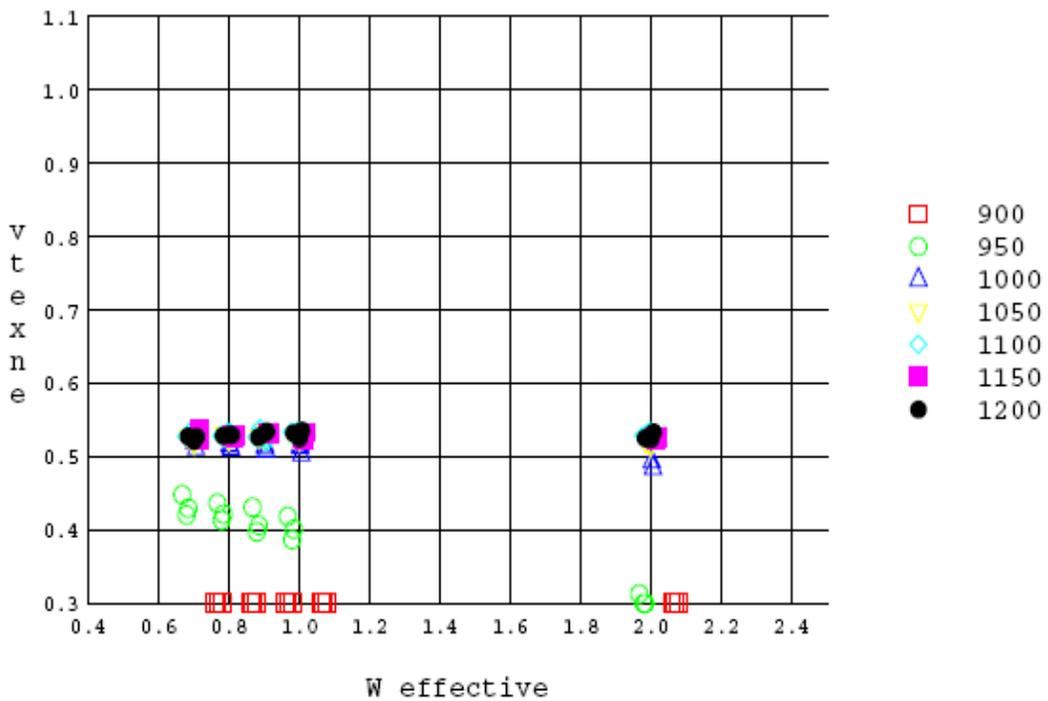
*Vt in HV NFET (high-voltage) for different field-implant resist thickness. HV part is very sensitive to the penetration of phosphorous (P @ 430keV) that occurs for resist thickness less than or equal to 1.050 $\mu$ m.*
