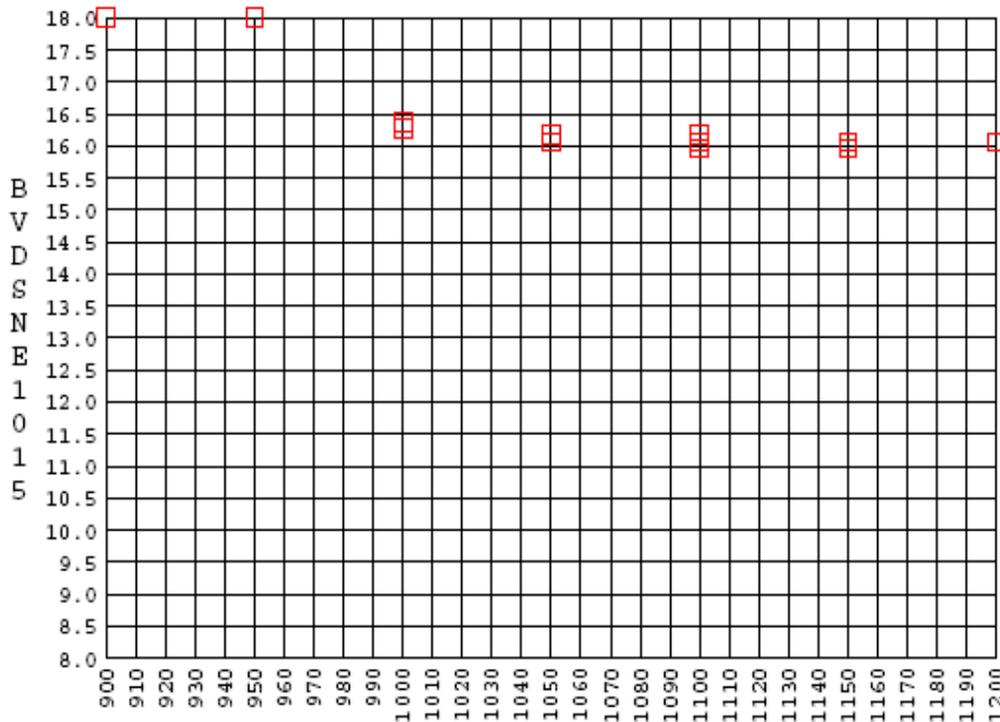
*Breakdown voltage of HV NMOST in EE block for different field-implant resist thickness (P @ 430keV). The penetration into the bulk occurs for thickness less than 1.050 $\mu$ m.*
