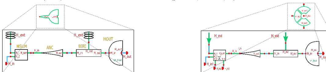
Fig. 2. Schematic view from Cadence Virtuoso depicting a nanomagnetic inverter model, comprising three parts: an ANC, a nanowire, and an output field generator. b) pNML majority gate, comprising the same main three parts as the inverter in a). Instead of one input, the majority gate has three or more inputs, depending on the type of device. All incoming fields are summed at the same instance and applied on the ANC. Each of the shown parts of a magnet is described in Verilog-A file.
