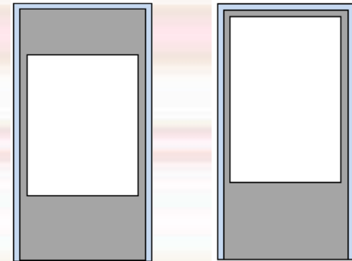
Schematic representation of 2D cut-plane of DG FinFET and trigate FinFET respectively
