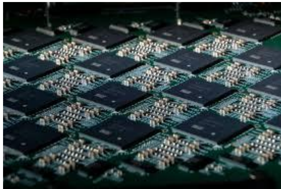
Server-scale neuromorphic HW: Loihi, Intel Labs
